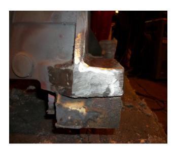
After the casting was completed, Metal Surgery X-rayed the casting. The X-ray came back with zero defects in the weld zone. Another success for Metal Surgery.
